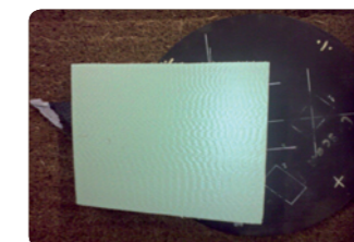
Heat insulation foam above CFRP:
