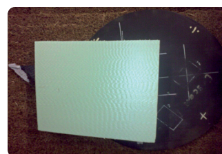
Heat insulation foam above CFRP:
