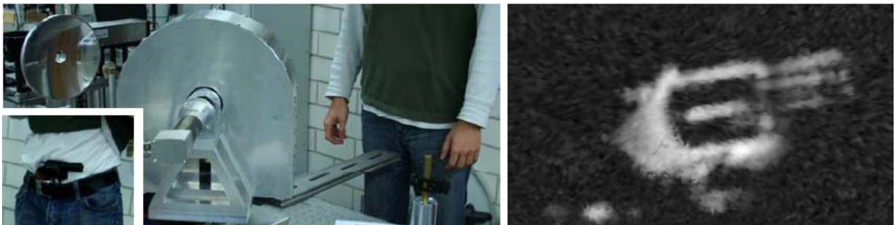
Figure 3: The good image quality is shown here; the hidden weapon can easily be detected. Please note that a real person is used to prove the real-world capability of the SynViewScan ROT system. Left: system setup. Right: The obtained Terahertz image.
